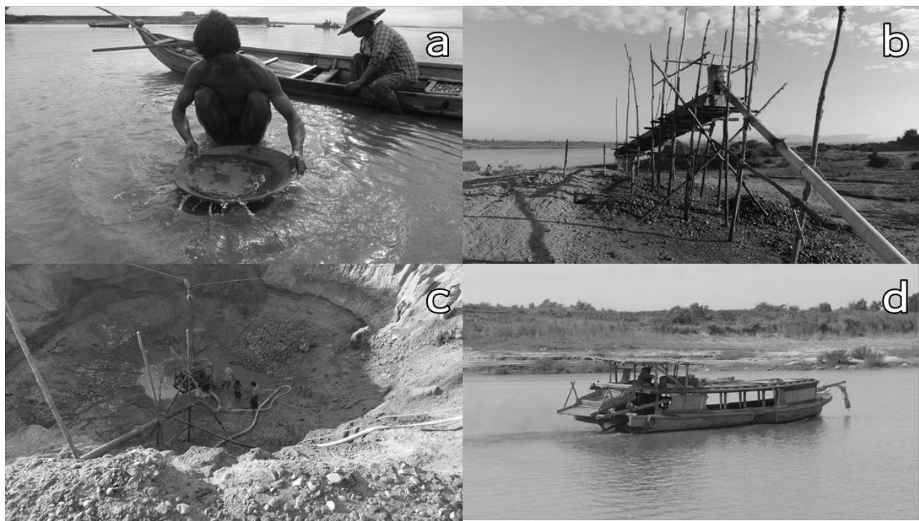
Fig. 2 Placer mining in the middle reaches of the Ayeyarwaddy River. (a) Gold panning in a river (*ta-naing-ta-paing ye-myaw*). (b) A wooden sluice with a water pipe (*si-phwa-phyit kone-myaw*). (c) A placer mining pit with a depth of over 10 m. (d) Gold mining boat (*si-phwa-phyit ye-myaw*).
